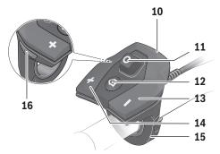
On the operating unit **10** you can set how much the eBike drive assists you while pedalling. The assistance level can be changed at any time, even while cycling.
